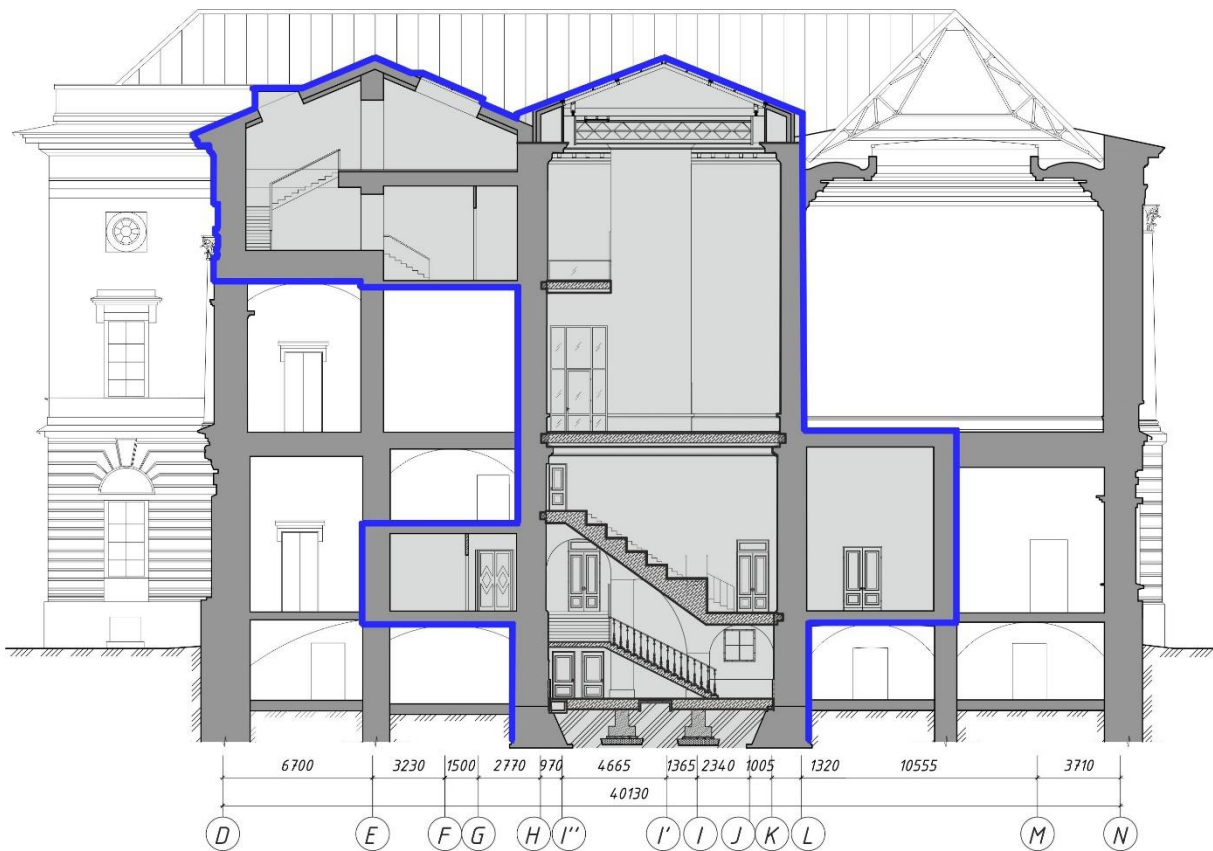
Figure 7 - A cross-section of the Western courtyard (AMS).
